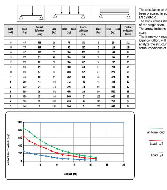
The calculation at the base of the table has been prepared in accordance with the UNI EN 1999-1-1.
