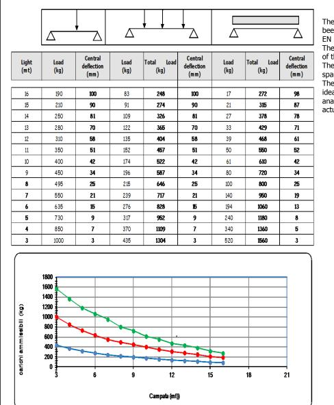
The calculation at the base of the table has been prepared in accordance with the UNI EN 1999-1-1.
